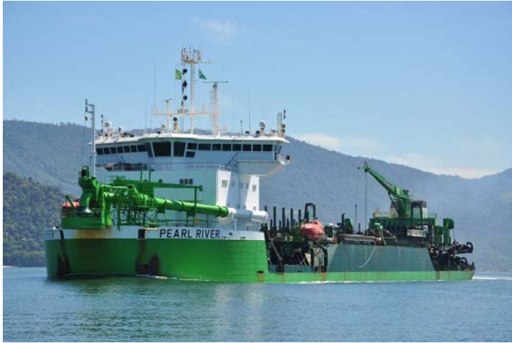
TSHD 'Pearl River' performing capital dredging works in Porto Sudeste, Sepetiba Bay, Rio de Janeiro in Brasil
