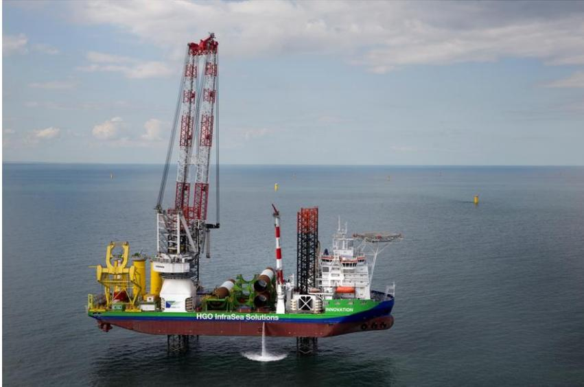
*GeoSea's jack-up vessel 'Innovation' performing installation works at Westermost Rough offshore wind farm, UK*
