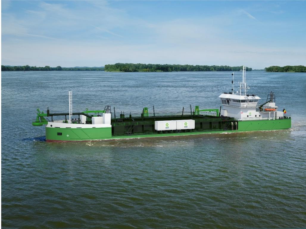
**Impression of the 2,300 m<sup>3</sup> trailing suction hopper dredger**
